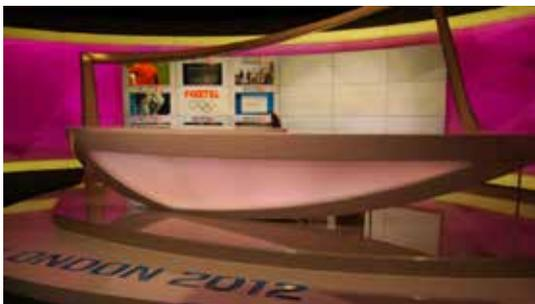
The smaller Silver Studio included a similar organically shaped desk with a large LED screen to the rear and a small, curved section of seating. This desk was also inset with LED lighting details and a back lit plastic panel. The steel and timber curved rear walls of the set incorporated graphics and the floor was given a high gloss finish. Features were highlighted using back-lighting and RGB LED colour changing trim and a 2pak high-spec finish was used throughout.
