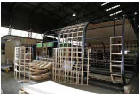
Time is probably the single most critical factor in every project we make. The structures for Android Works required curved steel yet the lead time was such that there was no time for the standard process of rolling or bending to the required radii. Instead, we cut profiles from steel plate creating structurally sound and strong box sections able to meet the specification of withstanding 100km/h winds.
